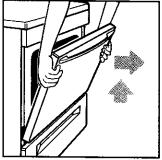
4. Pull door straight up, then toward you. Hinge hangers will slide out of front frame hinge slot.
